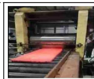
Hot Rolling Mill
