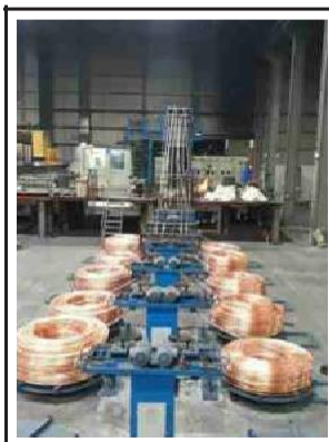
Vertical Casting Machine
