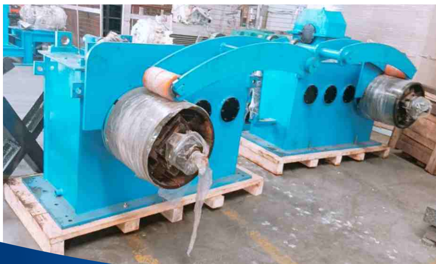
ROLLING MILL COILER DE-COILER
