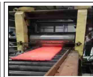
Hot Rolling Mill
